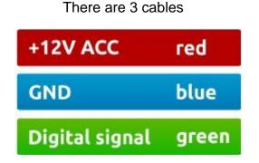
Before connecting the emulator, use multimeter to check signals on pins in the plug!
