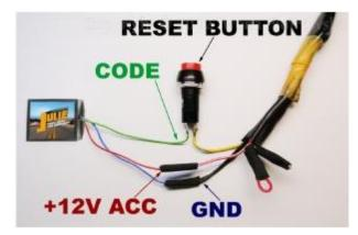
You connect code line by pressing the RESET button. In order to start the motorbike you firstly need to press and hold the RESET button, then turn the ignition and then release the RESET button. Now you can start the engine.
