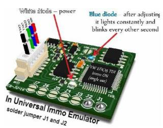
This emulator replaces damaged immobiliser, instrument cluster or a car key. Immo gets removed once the emulator is connected to the OBD socket. In the case of losing car keys or car theft, you will be able to drive to the nearest car garage
