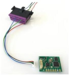
Connect all the wires to the OBD2 socket
