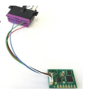
VW EDC15 emulator does not remove immo due to a program change to flash memory in ECU:
