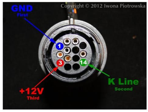
Fitting procedure of emulator is the same as for the OBD2 socket
