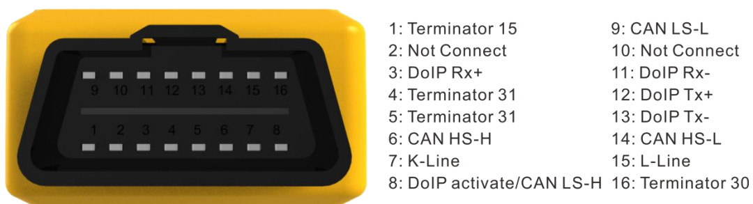
Fig2-2 SVCI 6154A Interface PIN Layout
