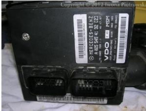
ECU is located on the air delivery pipe together with with Air Mass Flow Sensor
