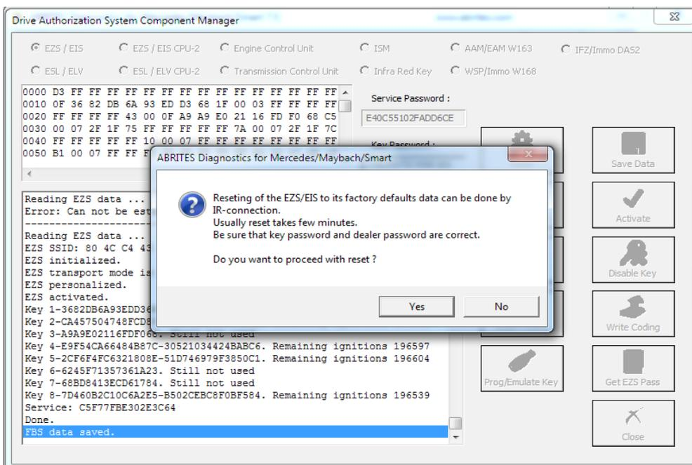
After confirming you can proceed to the next step. Do NOT forget to have your IR connector connected to the AVDI and ready to be plugged into the EZS when the software asks for it:
