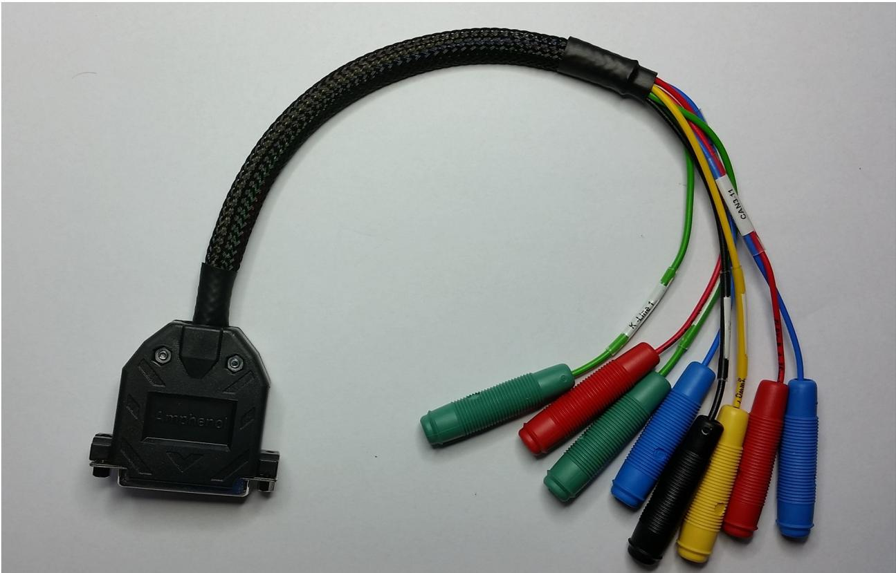
2. Abrites Switch Relay Cable. It allows the password extraction speed to be increased drastically when all keys are lost. It is used together with the Abrites Fuse Plug.
