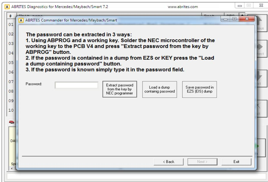
1. You can use Abprog programmer and solder the NEC MCU of a working to it in order to read the password from it. (explained in details in the message on the screen)
