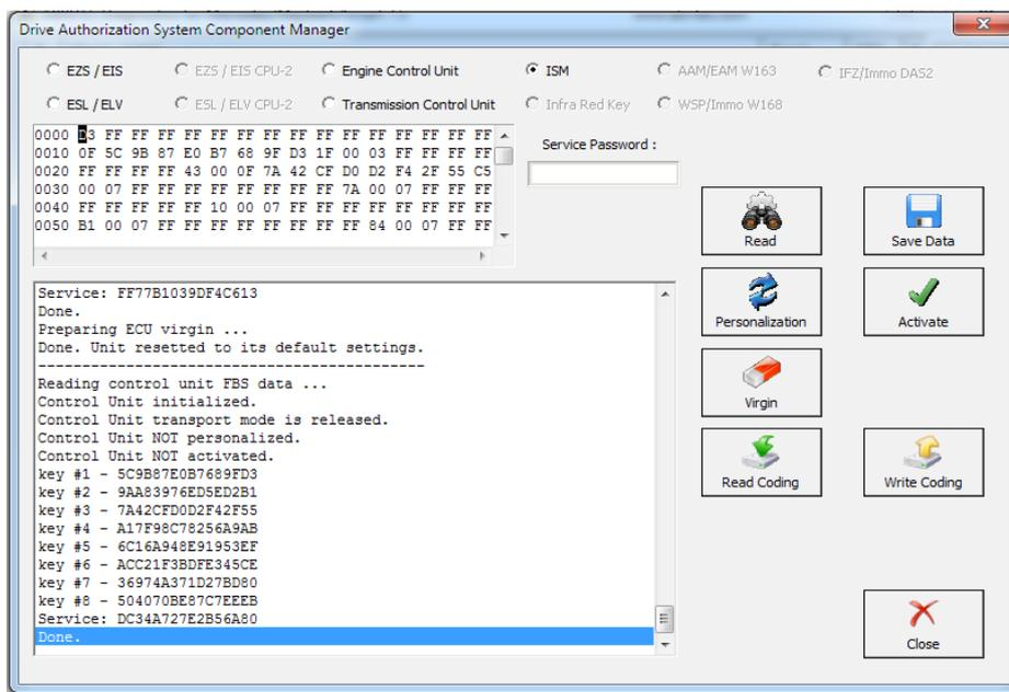
In order to personalize an ISM unit you have to either turn the ignition ON or reset the module. Now you can proceed. It is best to put the ignition ON:
