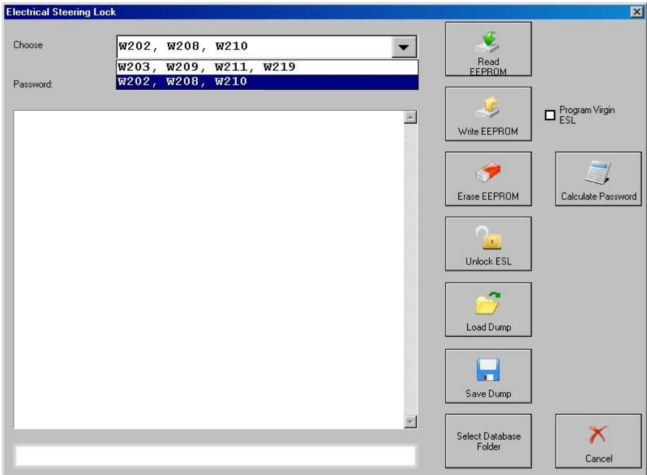
For some vehicles it is possible to replace the NEC ESL with a Motorola ESL. Such vehicles are Vito 639 and Mercedes Sprinter 906.
