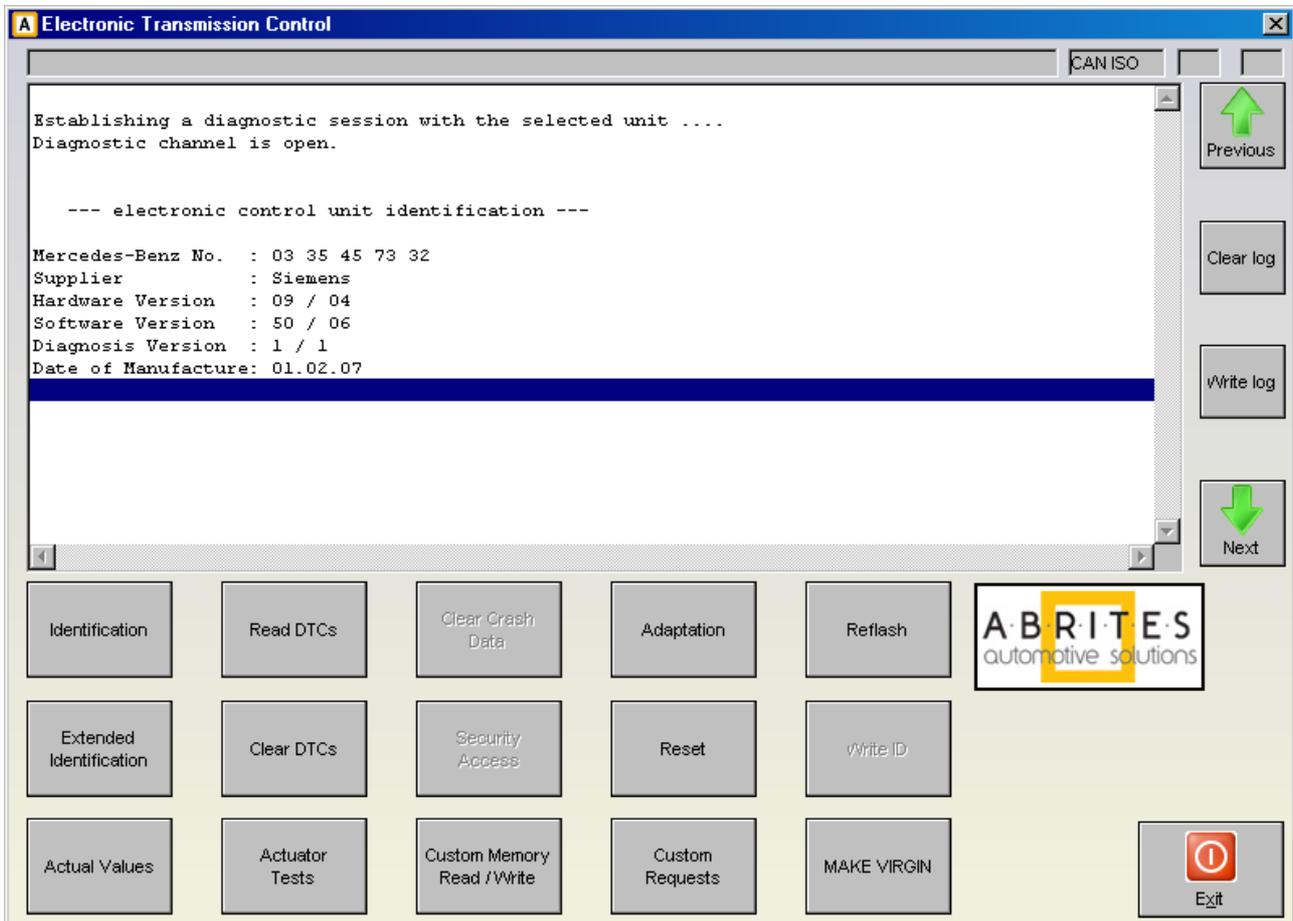
1.3. Pressing the button “Adaptation” will show the available adaptations including the SCN coding string. You may save the SCN coding string from a damaged control unit and then you can save this saved SCN coding in the donor 722.9 control unit:
