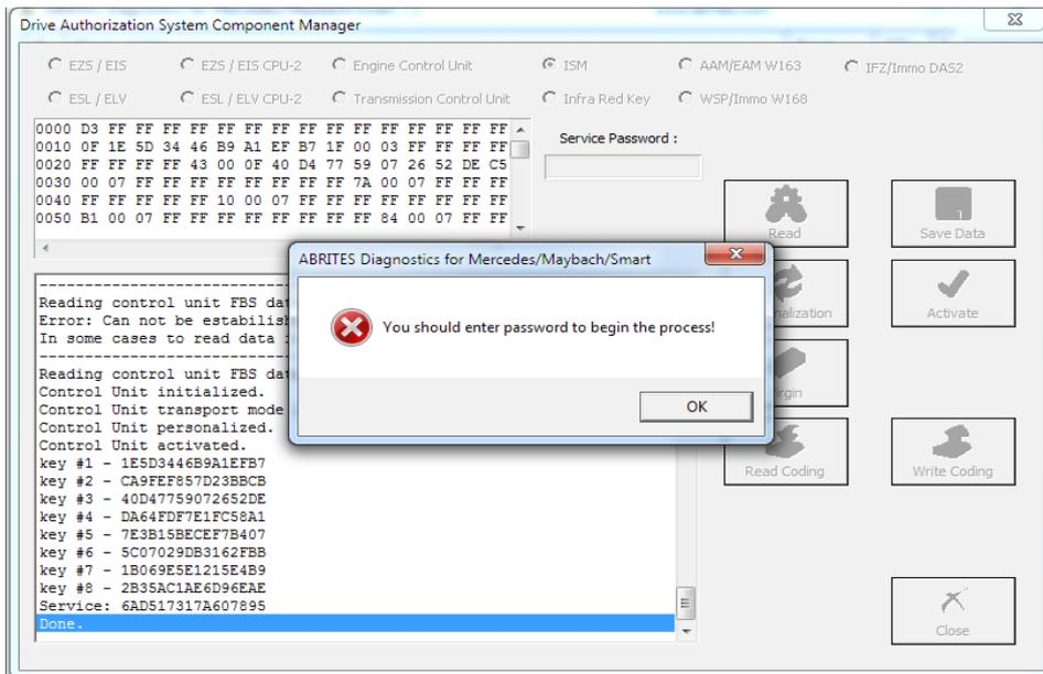
Once the service password is calculated the ISM can become virgin. This needs to happen inside the car via internal Can or outside connected on a bench rig. Also once the password is saved to your computer – you can use it indefinitely:
