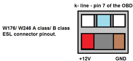
For most models it will be a direct plug in, but in the case of the W204, W207 and W212 for example you need to follow a procedure to perform the ESL emulator adaptation once you have the Key password. The EZS needs to **be read, then press SAVE DATA (this is the FBS/DAS data), save the data**, then make sure to save the coding and know where they are on your computer
