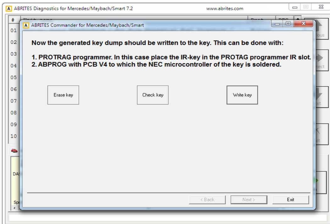
1. Using the PROTAG programmer's IR port. An IR key needs to be placed in the IR key slot of the programmer.
