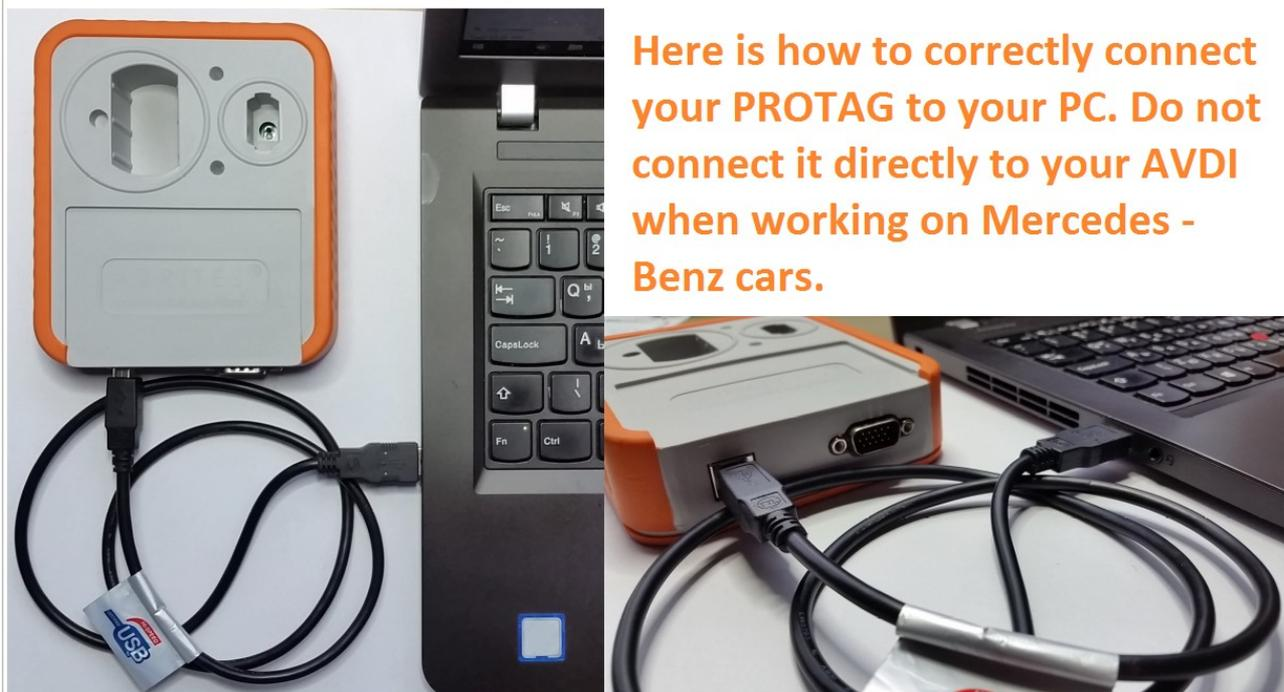
Here is how to correctly connect your PROTAG to your PC. Do not connect it directly to your AVDI when working on Mercedes - Benz cars.
