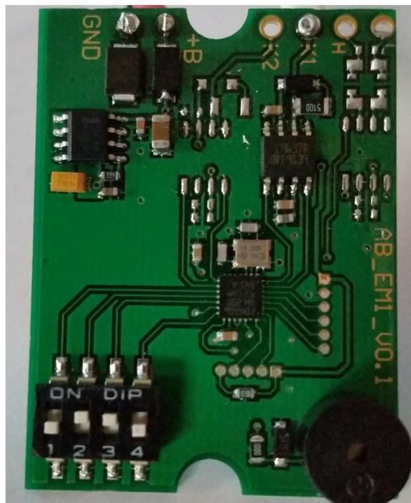
In the bottom left of the emulator you can see the switch board which is used to select the model you are working with.
