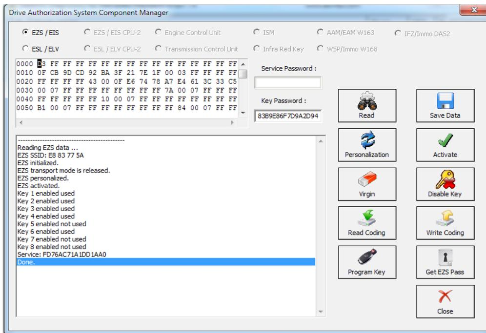
The procedure can also be performed with the ZN036 attached to the AVDI via the ZN030 and your Protag programmer attached to your computer. Please note that you will need to have internet connection to the laptop computer. You can read the password from the existing key (BGA type as well).
