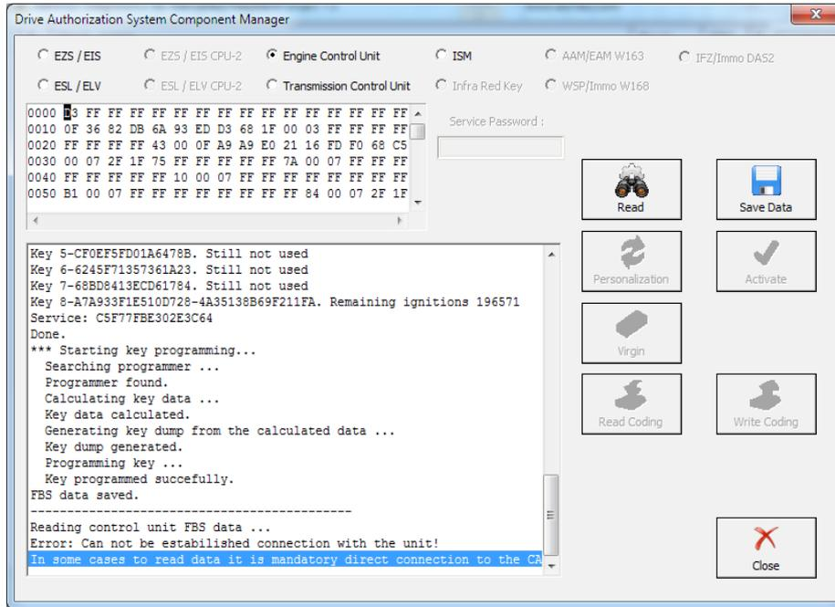
After connecting to the internal CAN we can retry the reading process. The following will appear:
