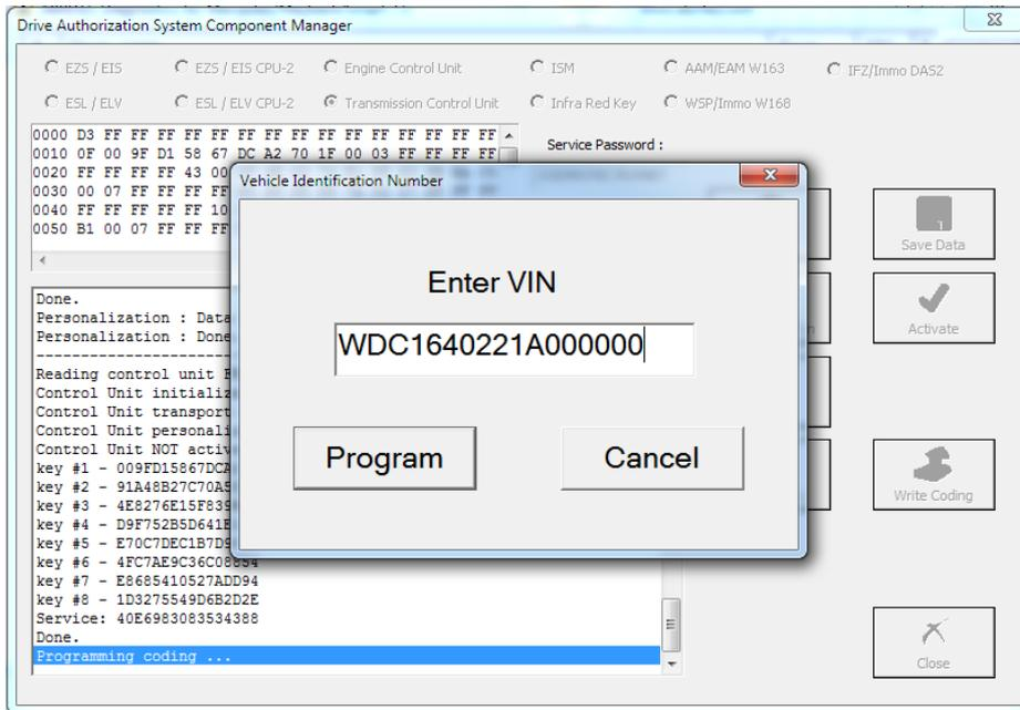
After that you can perform the latest step which is the activation. After that the TCU is ready to work in the car:
