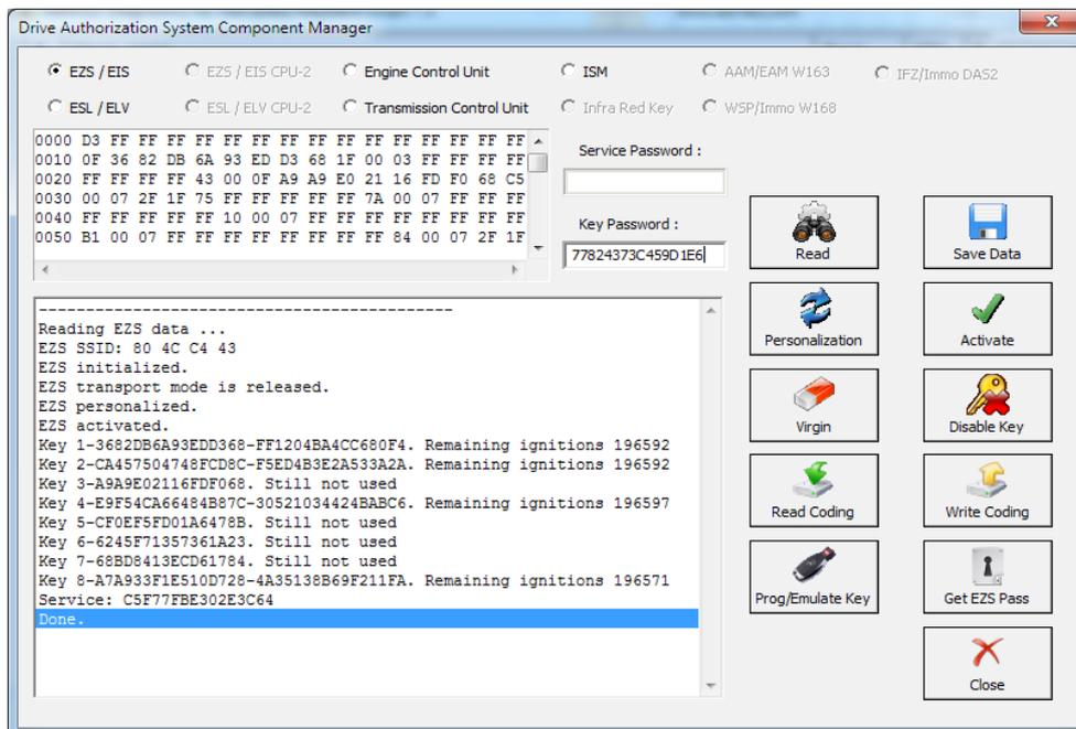
When the key password is added you can Program an Abrites key with PROTAG or Emulate a key with your IR adapter:
