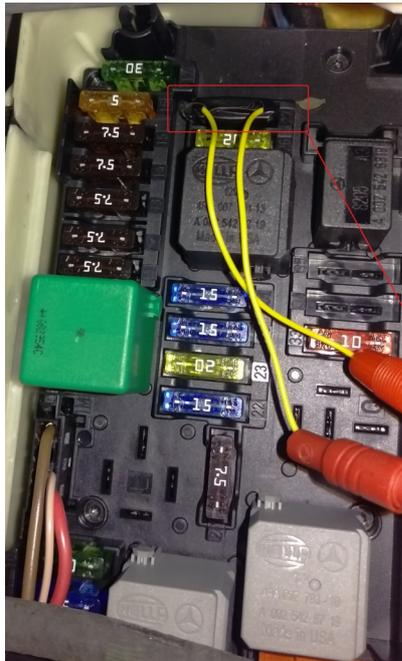
When working on a W204 car for all keys lost for example you can open the front SAM module on the driver side and see fuse number "27" - disconnect it, connect your ABRITES FUSE RELAY CONNECTOR and plug your relay and proceed to start the All keys lost procedure. Make sure that the ZN036 is in the EZS and that it is in the ignition "ON" position.
