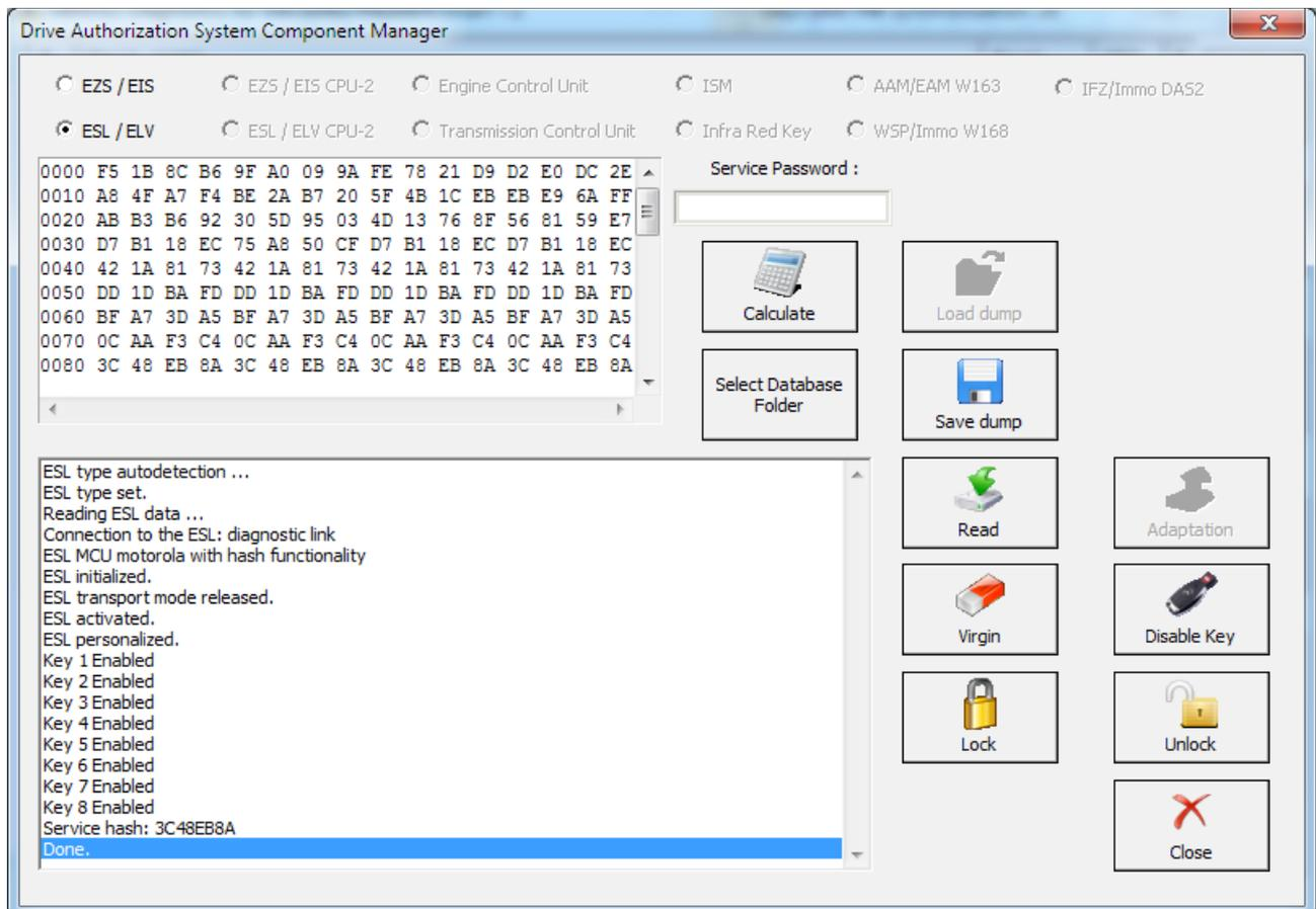
Using the options from the list you can perform all needed adaptations to the ESL/ELV. With this option you can also reset, unlock the electronic steering lock, make it virgin, extract the service password and many other functions.
