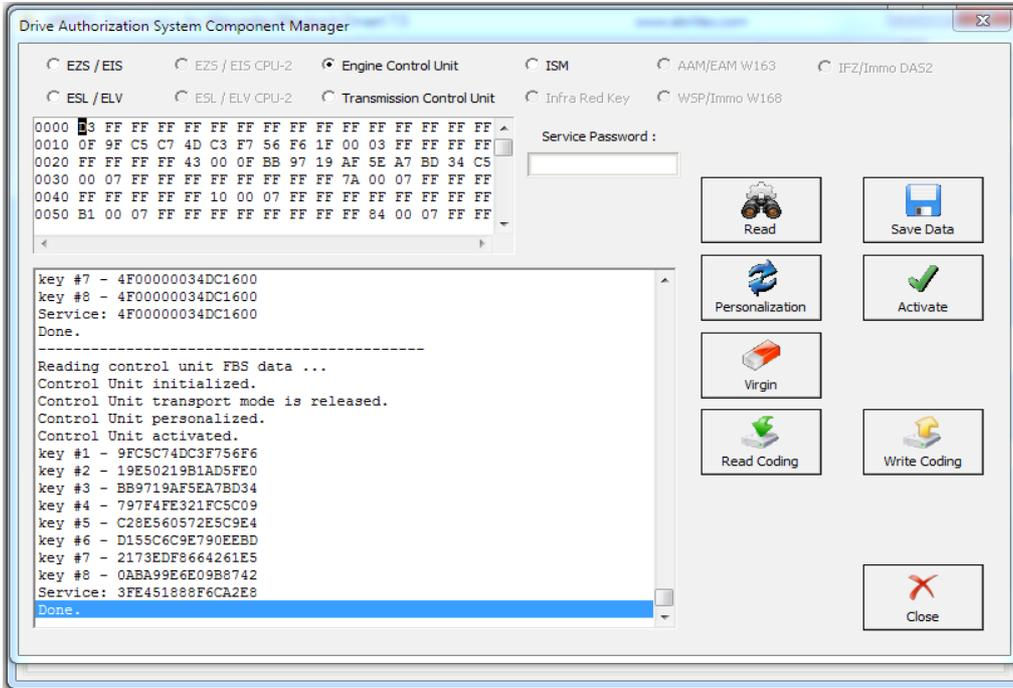
2. The used ECU is in a virgin state. You can turn the ignition OFF and ON again. Then press personalization:
