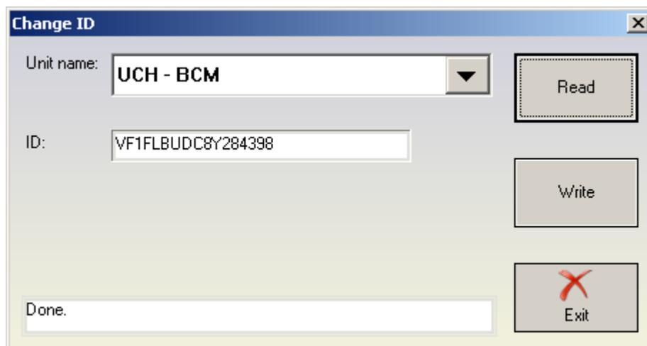
For each device you can try to read and change the Vehicle Identification Number. When changing this number there is also a checksum which is calculated automatically.
