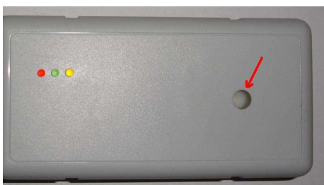
Fig.4 transponder place (old Hitag2 programmer)
