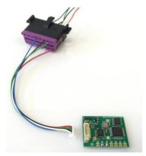
1. Connect all the wires to the OBD2 socket
