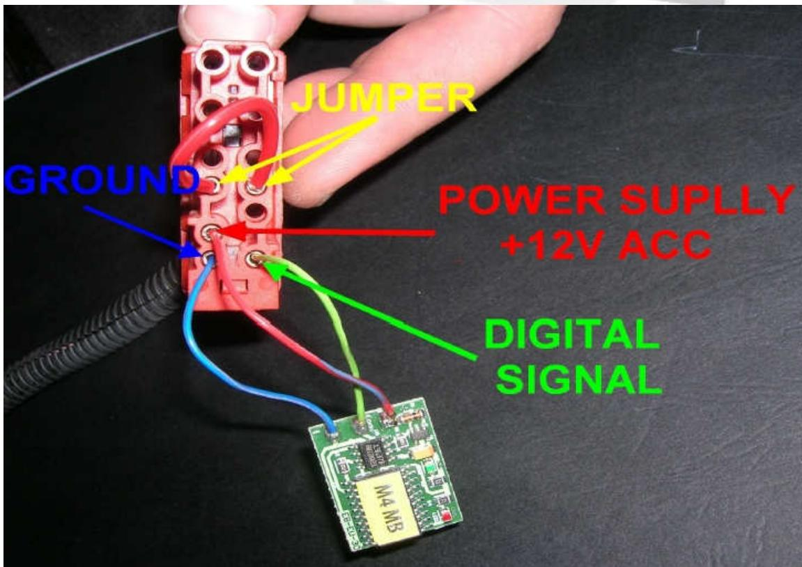
**After correctly connecting the emulator, error SRS/AIRBAG on instrument cluster goes off, without necessity of deleting code of flaws.**
