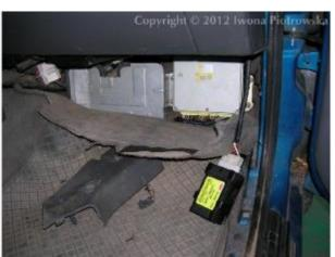
ECU is located under the floor mat at the front of the passenger-side footwell.
