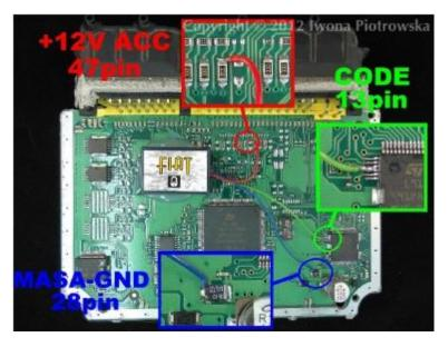
Cut off pin 13 from wiring in the car !!!
