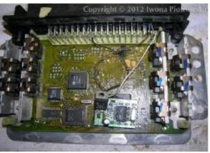
Connect immo line to **pin 55**. Disconnect immo. Connect A6 and A5 together.
