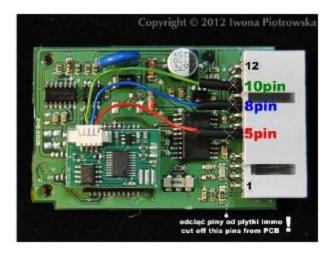
Connect emulator to the socket of disconnected immobiliser:
